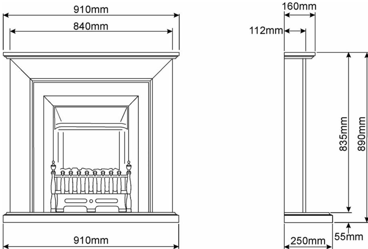
Figure 2. Dimensions (Heater shown for illustration purposes only)
